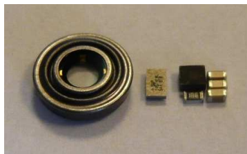
Figure 3. Liquid lens and driver MAX14574EWL+ with external components
