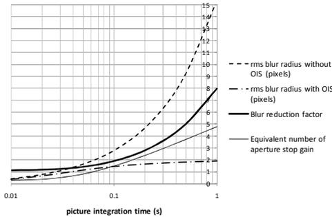
Fig.1. Performance evaluation of OIS system with A316S liquid lens
