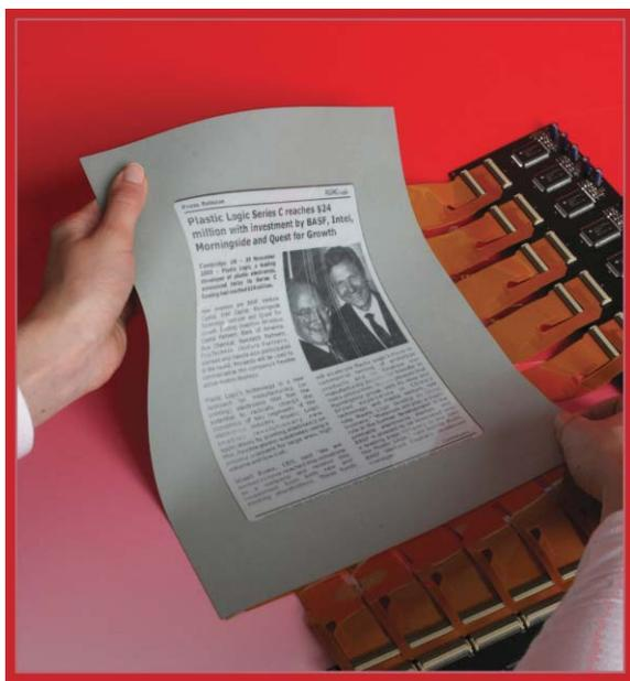
**Fig. 12** Realization of the use of electronic paper for reading a newspaper. This is an archetype of Plastic Logic Co. based on microcapsule technology.
