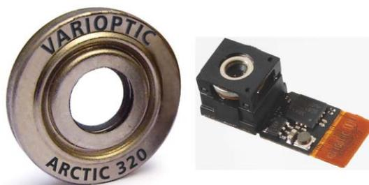
**Fig. 8** Electrowetting variable focus liquid lens. Left: A miniature liquid lens inside its metal case. The case diameter is 10.5 mm. Right: The same lens with its electronic control as is used for digital cameras in mobile phone applications. Courtesy of Varioptic Co.
