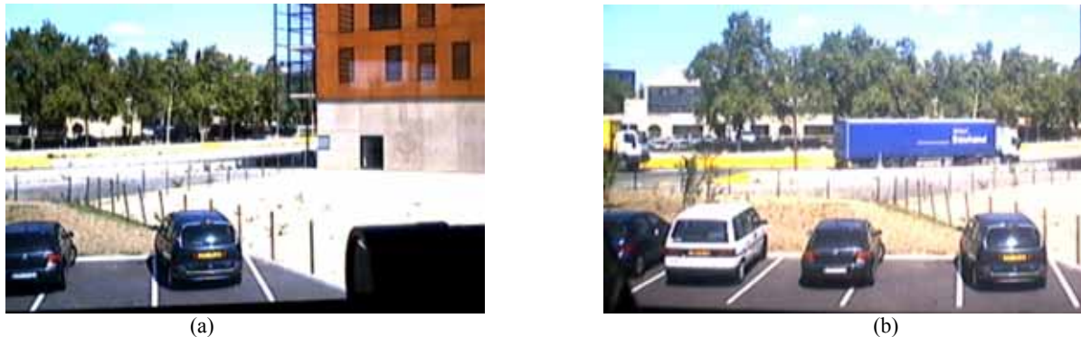
Figure 7: Image for an infinite object distance by a demonstrator (a) without and (b) with variable lens
